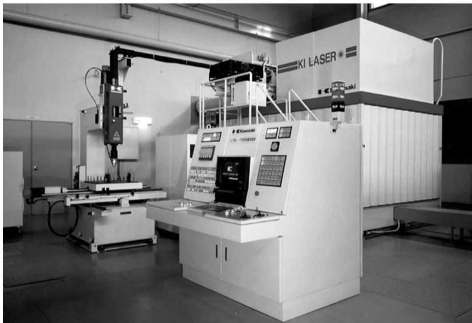
FIGURE 9.10 Photo of Kawasaki Heavy Industry's chemical oxygen iodine laser (COIL) welder. (Courtesy of Dr. Fumio Wani, Kawasaki Heavy Industry, Gifu, Japan. With permission.)
